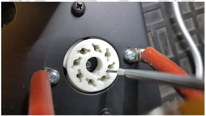
Please make sure you don't close these pins up fully or it will be difficult to replace the Valves. Replacement valve kits including tools for biasing such as a Multimeter and Terminal Screwdrivers are available directly from the Victory shop. Please visit <a href="https://www.victorystore.co.uk">www.victorystore.co.uk</a> for spares, accessories and clothing.
