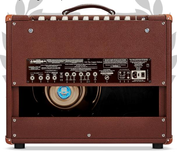
All rear panel sockets & facilities are mirrored on a screened rear plate so they can be easily located. This plate needs to be removed to reveal the 2 x M6 hidden amplifier fixing bolts for when the amp section needs to be accessed. The entire amp section is screwed to a wooden panel with 4 wood screws. Please remove this
